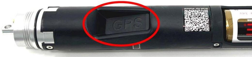
Instruct the AquaTel® unit to calculate and store the current position by sending the **PO** command by SMS. This is the position command.
