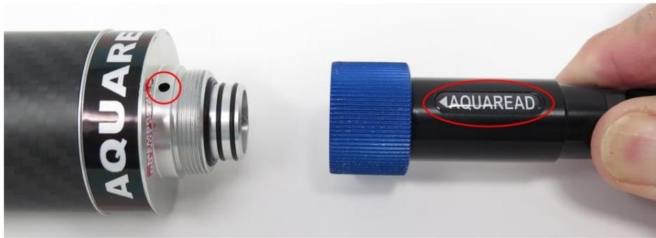
If you are planning to connect an external power supply, this should be done later. For the purposes of proving the system, connect the sonde/probe directly to the unit.
