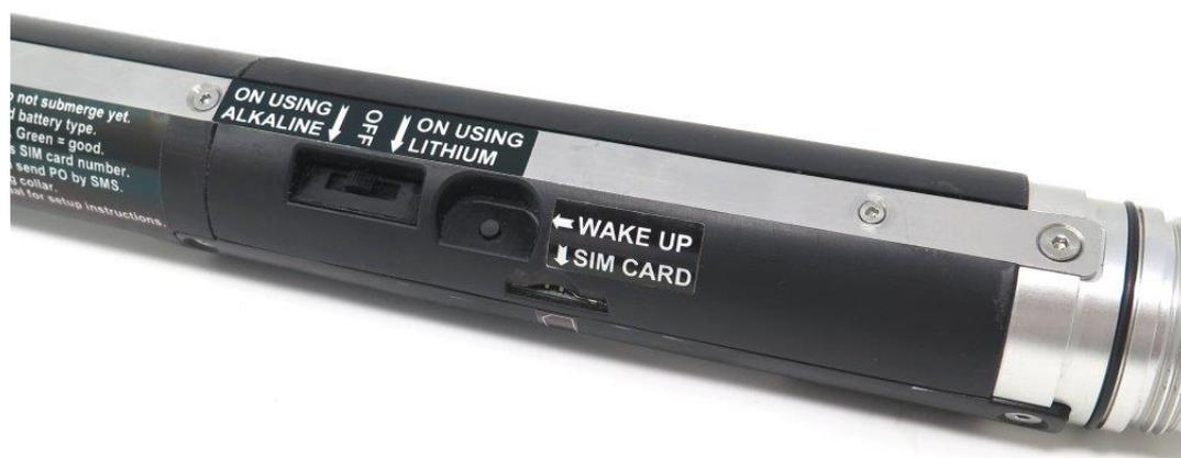
Insert the micro-SIM card into the slot marked 'SIM CARD' orientated as indicated by the graphic below the slot. The card should click into place. To remove the card, press it in, and it will pop out.
