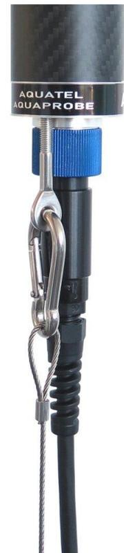
The AquaTel® unit is designed to be used outdoors and is rated to IP67, it is waterproof, but it **is not** designed for full submersion. You may notice a small hole on the base of the unit. This is a waterproof vent for the internal barometric sensor. **Do not poke anything in this hole!** Doing so will cause major damage to the vent's waterproof membrane and invalidate your warranty.
