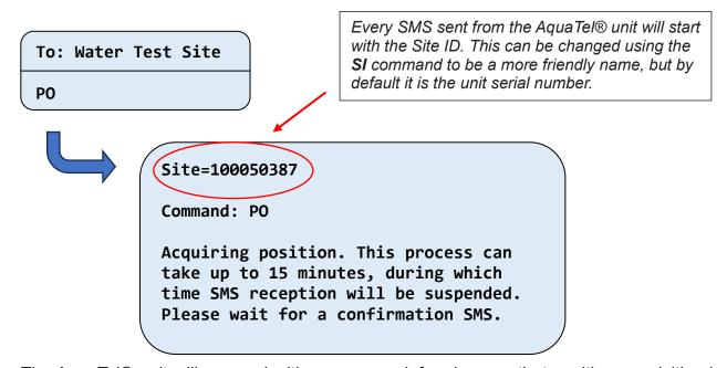
The AquaTel® unit will respond with a message informing you that position acquisition has begun. This procedure can take up to fifteen minutes. As soon as the position has been established, you will receive a confirmation SMS, which will include the latitude and longitude for the unit's location.
