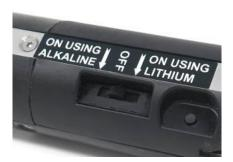
It is very important that the switch is set at the correct position for the battery type in use.
