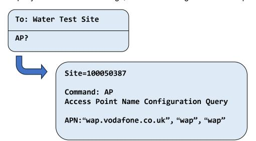
If you are not sure what to enter for the APN, please contact your SIM card provider. In many cases using the default APN will work correctly. However, if you have issues with the FTP data upload or local time settings, it is likely that the APN needs setting for you SIM card.
