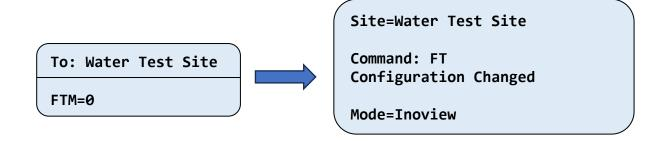
For full server details, send the FT? command to the AquaTel® unit by SMS.
