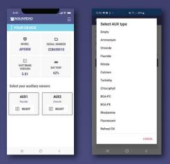
Within the Your Device screen information about the Aquaprobe is displayed. Including serial number, software version and the remaining battery level of the Bluelink device.
