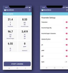
Displayed on the Live Data screen are all of the currently measured readings coming from your connected Aquaprobe.
