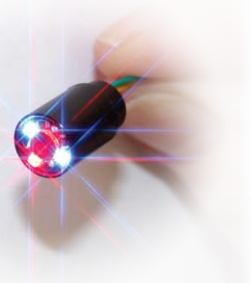
Optical DO sensor LED's flash during measurement.
